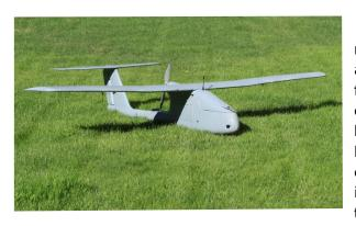
The plane is based in COTS materials (Commercial off-the-shelf) and has been adapted to became a complete UAV. Due to the fact than the plane has been built using composites and EPO its weight is really low(1.3 kg without the payload) it is really easy to hand launch it and to land it: any operator can do it, even without any previous skill, and it will land on its fuselage without big damage in almost any terrain. UAV Remote Sensing Skywalker.
