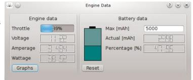
The system also monitors the amount of energy that came from the batteries and uses the batteries up to the point it is bingo time. Batteries packs are available from 5.000 mAh to 13.000 mAh
