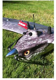
Its fuselage made of Kevlar® and Carbon Fabrics with Epoxy resin for the Aerospace Industries provide, together with the EPP wing, a high level of ruggedized to this UAV.
