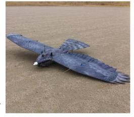
any previous flight experience and it is not even necessary to have a manual joystick because the system can fly 100% in automatic mode: from the take-off to the landing. In case of a communications problem the plane will came back home and land safely.
